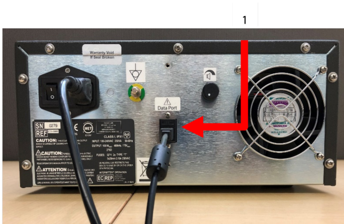
Figure 12: Atricle CS-3000 RF Generator Rear Panel with Data port (USB or Serial) (Image for reference only)
